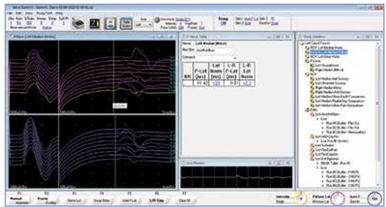
Automatic cursor placement and **Left vs. Right comparisons** in NCV, F, H, and Evoked Potential test protocols. Live Monitor window facilitates identification of artifacts or poor electrode connections. On-line comparison to reference data and identification of abnormal values. Unlimited number of traces displayed per test protocol.
