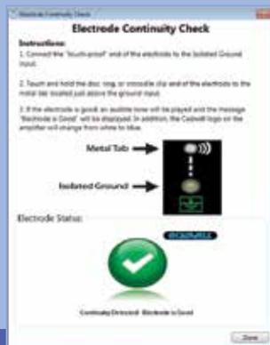
A unique electrode continuity check (Electrode Check) is built into each amplifier, so you can easily confirm if one of your electrode leads is good or bad.
